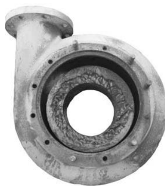
Figure 1.2.5.c: Results of abrasive fluid cavitation
