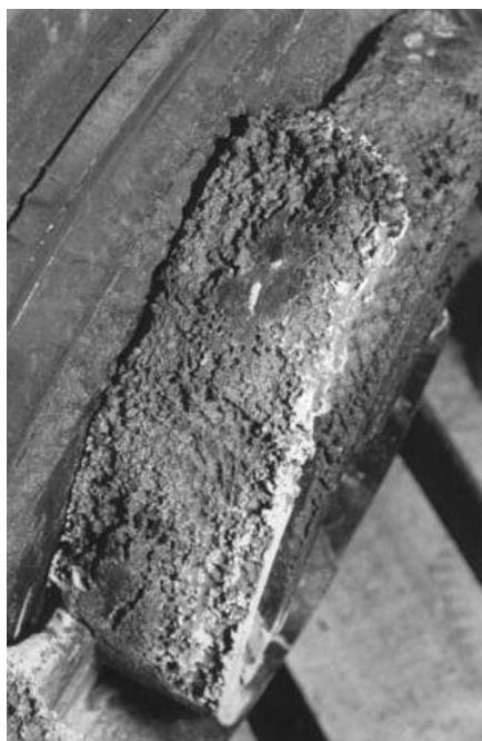
Figure 1.2.5.a: Results of clear fluid cavitation
