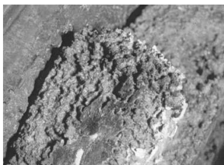
Figure 1.2.5.b: Results of clear fluid cavitation
