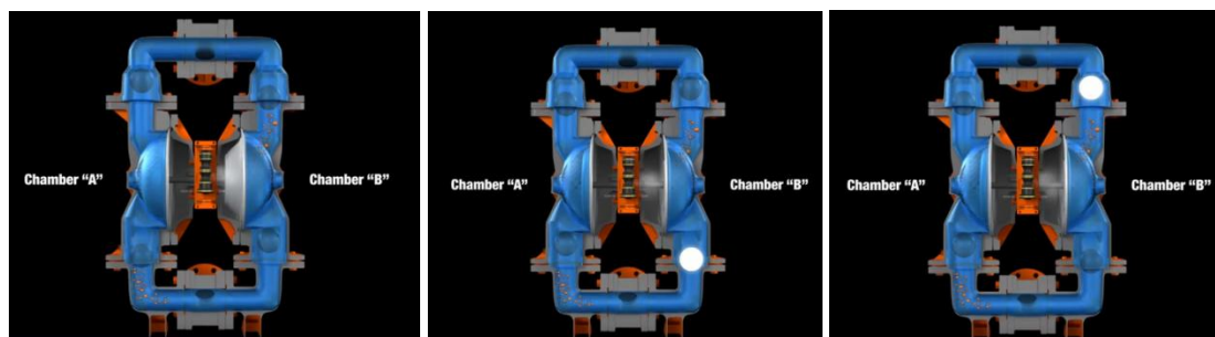
Figure 1.1.4.1.c: Hydraulically actuated double diaphragm pump
